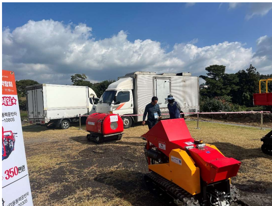
Fig 11 - Remote controlled mulcher and sprayer
